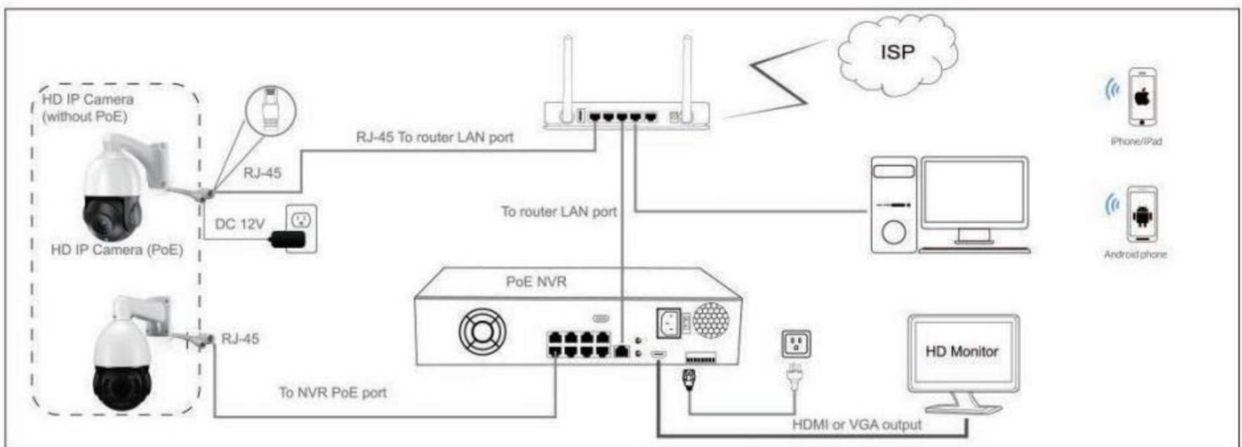
Figure A: Working with POE NVR
