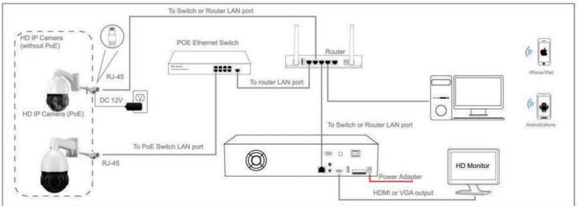
Figure B: Working with POE Switch
