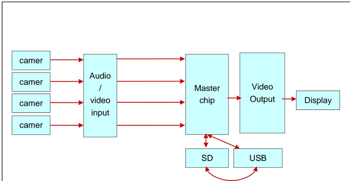
Monitoring system block diagram
