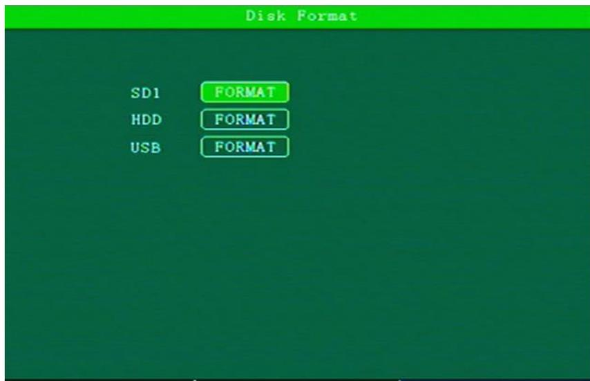
Format the SD1, HDD and USB , press the [ENTER] key.
