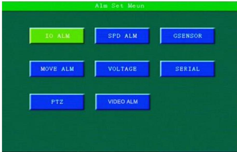
The menu contains IO alarm, speed alarm, acceleration, motion detection, alarm voltage, serial port management, PTZ control sub-menu. Press [ENTER] key to select.
