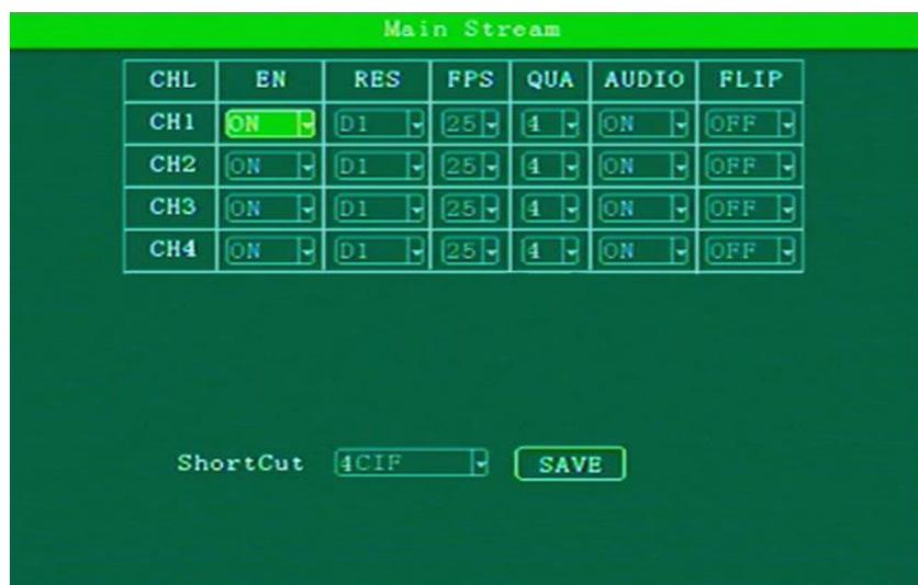
1/2/3/4 channel can be set individually, or you can set up quick, that the following shortcut options, while the four-channel set to CIF, HD1, D1, 720P, 1080P, press the [ENTER] key to select.
