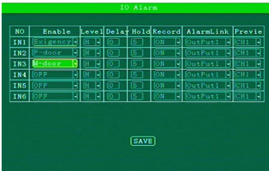
It supports up to 6 alarm input simultaneously. Set the alarm input, output and alarm recording parameters:
